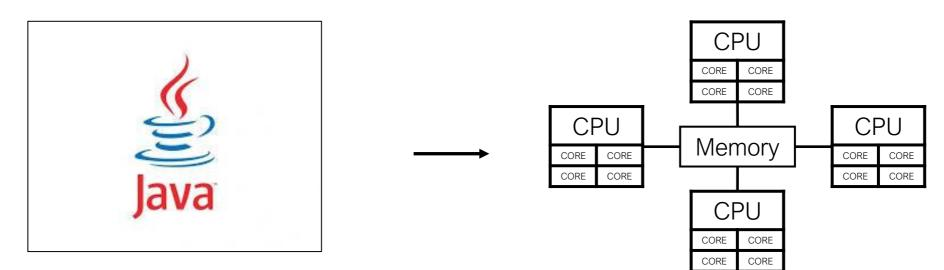
Multi-threaded, task-parallel applications executing on a single JVM A single shared-memory multicore machine
