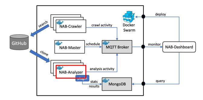
**NAB-Analyzer:** clones code from repositories, builds code, runs DPA on executable workloads
