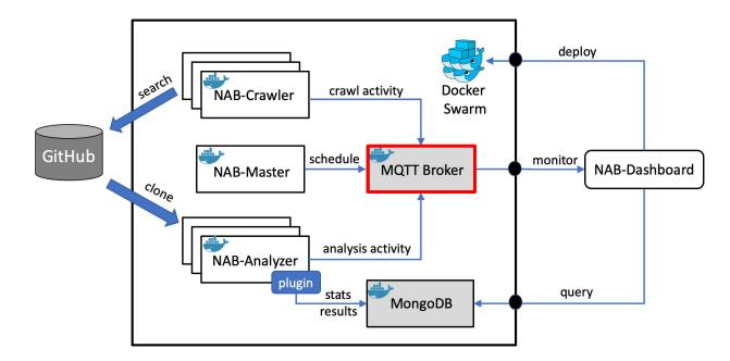
**MQTT Broker:** handles asynchronous communication through events (publish-subscribe communication protocol)
