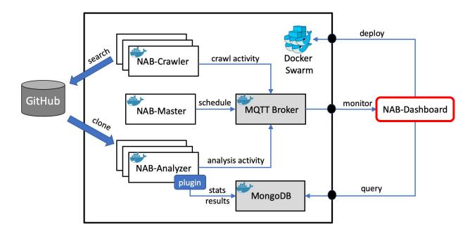
**NAB-Dashboard:** handles deployment of NAB services (using Docker Swarm), allows users to monitor DPA progress
